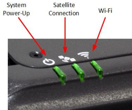
Figure 3-6 System, Satellite and Wi-Fi Status LED's
