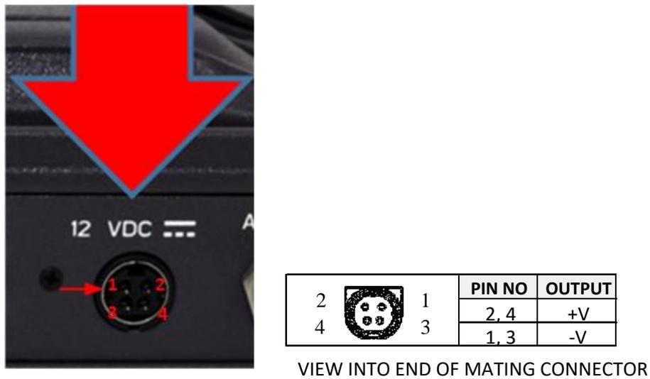
Figure 7-3 12V Input and Mating Connector Detail
