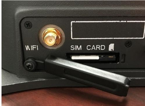
*Figure 3-3 SIM Card with Cover Opened*
