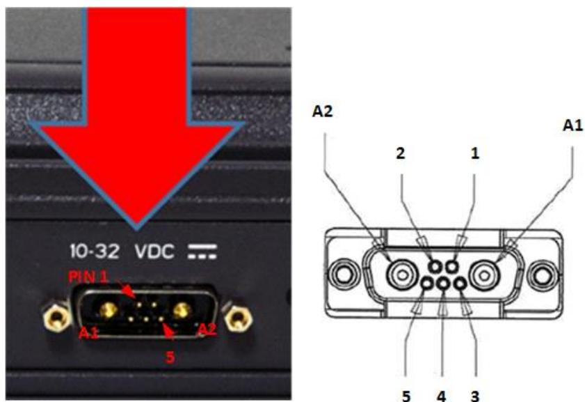
Figure 7-4 10-32 VDC and Mating Connector Detail
