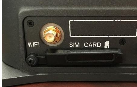
Figure 3-5 Secure the SIM Card Cover
