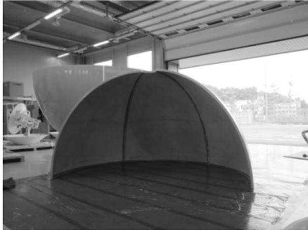
A. The assembly of the upper radome panels should now be completed, using the M6 x 35 bolts supplied.
