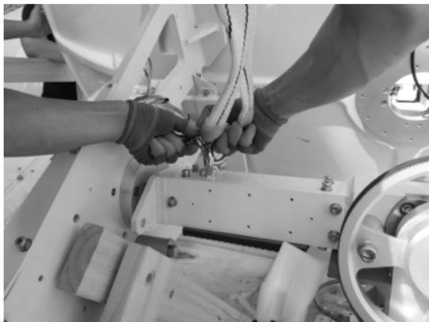
G. Securely hook the lifting straps as shown. (On the both side of the CL arm)
