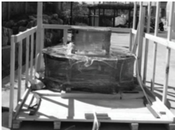
B. After complete removal of the wooden bar in section A directly above, the packaging should be seen as shown left.
