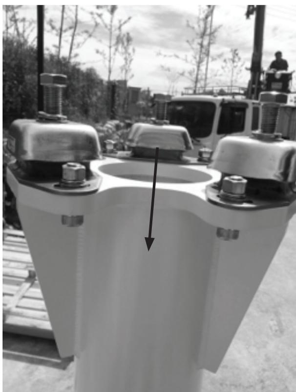
Check to confirm the orientation of the pedestal support with regards to the bow.
