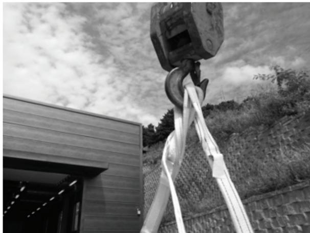
B. Secure the strap tightly as shown left for a safe removal.
