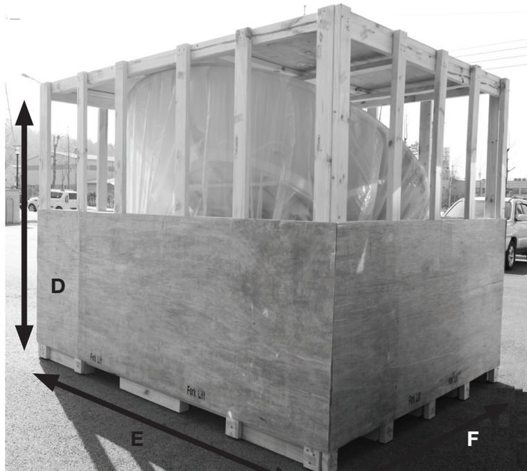
To secure the safe installation process, please make sure to have enough space (10m x 10m x 10m) around the unit
