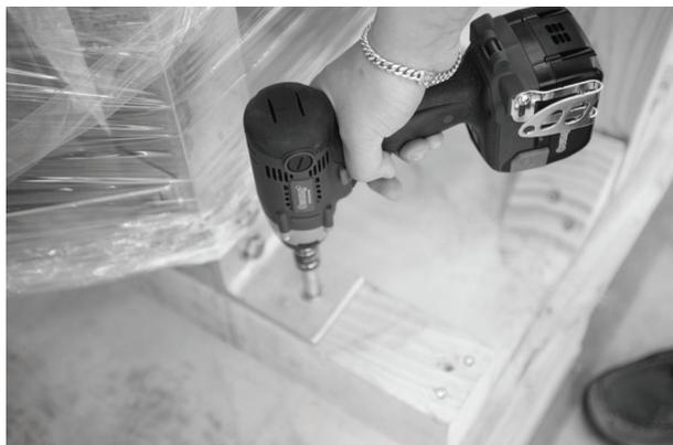
C. Now prepare to remove the Base frame by removing bolts from wooden crate floor and base frame legs.
