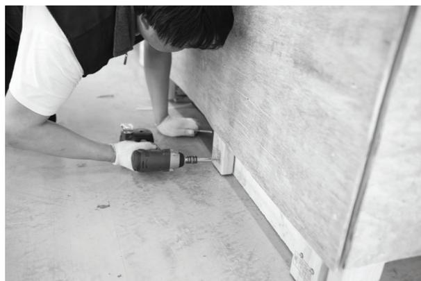
C. The packaing will be taken apart using an Impact Drill.
