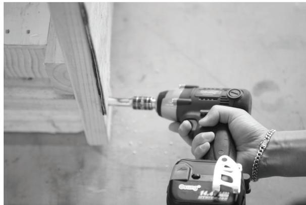
B. The packaing will be taken apart using an Impact Drill.
