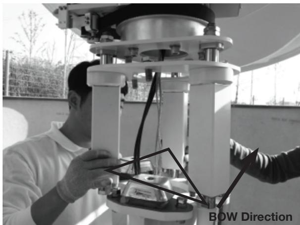
A. Locate the power and RF cables as shown.
