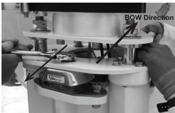
B. Insert the 3 M16 x 40 bolts to secure the antenna assembly to the pedestal. Make sure to apply Loctite 262 to securely tighten the assembly.
