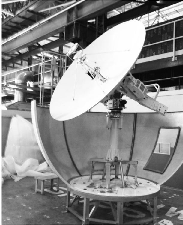
A. Assemble 5 radome panels as indicated in previous section.
