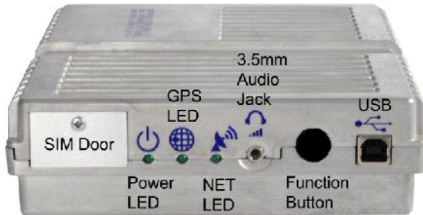
Figure 1-6 – Front side view of IDU
