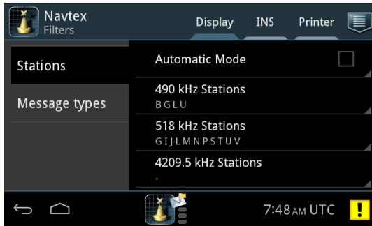
Figure 11: Filters for stations
