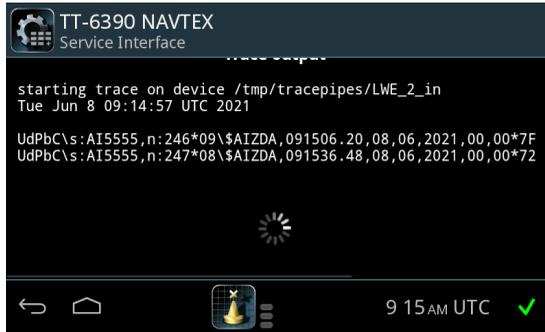
Figure 21: Service Interface, NMEA trace ongoing
