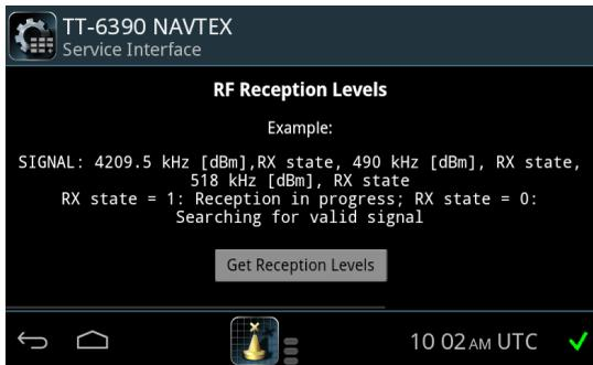
Figure 23: Service Interface, RF reception levels
