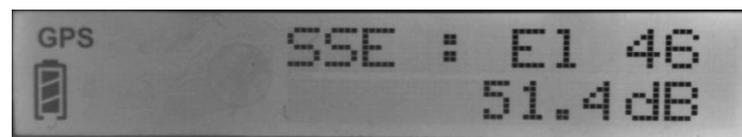
Use the signal quality bar and numeric display on the lower line to help point the UT to the satellite. While in pointing mode, you may also activate the audio pointing aid by a long press of the audio button on the right.
