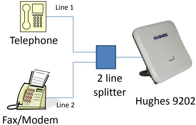
1. The Hughes 9202 RJ14 port allows the connection of both a telephone and a fax or modem at the same time (BGAN circuit switched network restrictions mandate that only one is in use at any given time).
