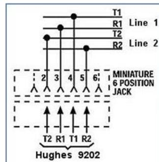
Note: with release 5.8.3.0 and higher, if you have a device that supports both voice and 3.1kHz/fax with a single line, you can configure the RJ14 port to support both services on line 1. Refer to the Telephony section.
